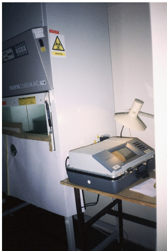
Fig. 1. Photograph of the Laser Fiber Monitor (right) connected with the AURA Cabinet (left), here adapted for the fiber emission experiments.
